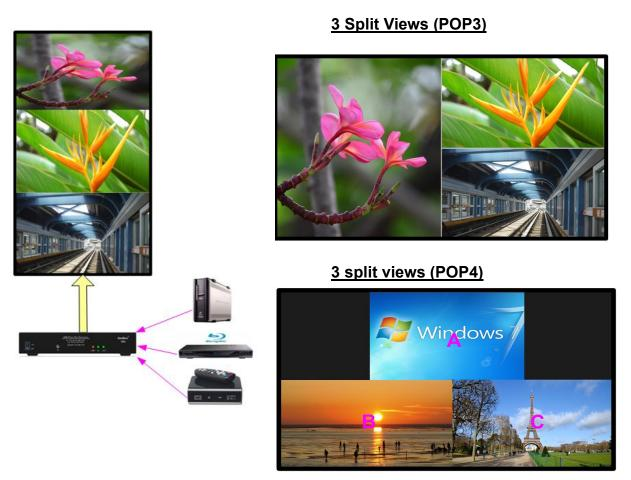
User can swap the RH/LH images on POP3 and Top/Bottom images on POP4 by image rotation and change the monitor installation direction (top/down direction). Aspect ratio in each window is adjustable.
