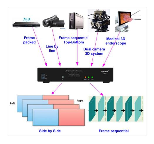
User can apply dual camera FHD 3D signal to G901. G901 can be set at POP SBS mode and output 4k/2k side by side image for 3D display.
