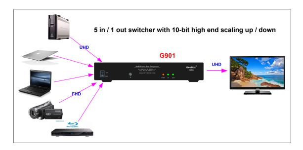
(5x1 seamless switcher. No any frame loss to prevent projector from spending time for re-search input source)
