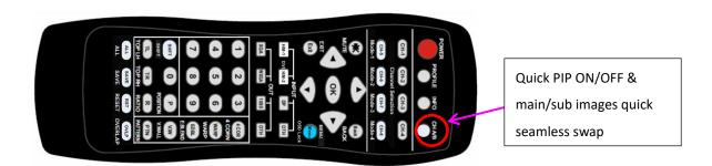
➤ User can assign one input to main image and another input to PIP image with full PIP size and set G901 output resolution at FHD, then click [CH A/B] key to execute seamless quick swap between these two inputs.
